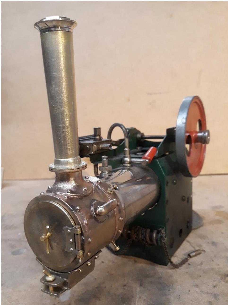
Before final assembly line up the holes on the chimney base plate with the chimney itself and secure with the 6 x 12BA bolts as supplied
