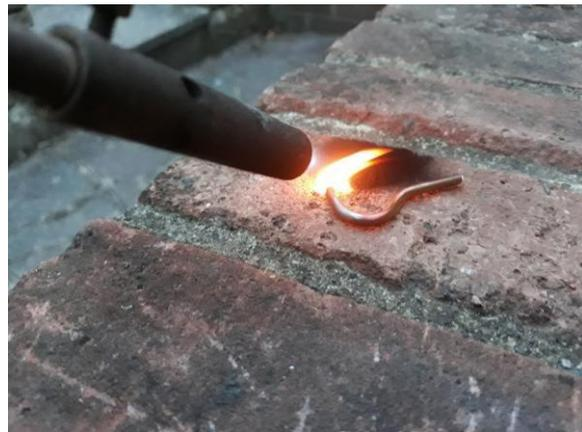
One neat dodge is to fabricate the pipework you need with an offcut of 2.5mm mains cable as a guide and form your pipework to this as a template.
