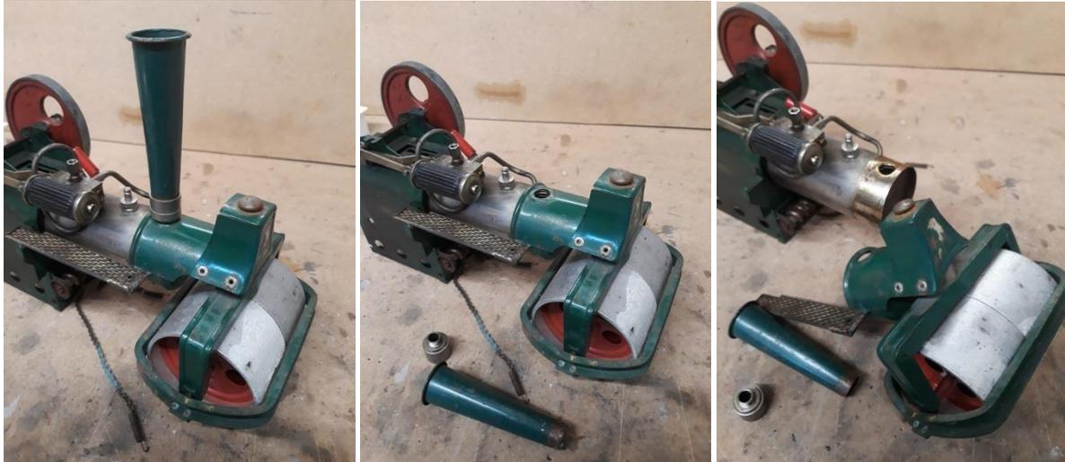
... drill out the rivet holding the checker plated footboard to the smokebox bracket. It's a good idea to refit the footboard as this acts as a drip tray for the cylinder.
