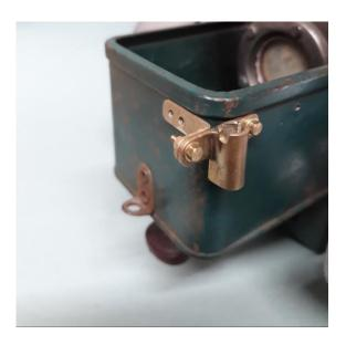
You know have the option of (1) or (2) if you require the canopy fitted then remove the bracket and fit the seat support to the side and drill the second hole in the tender side, bolt this in place and that's finished
