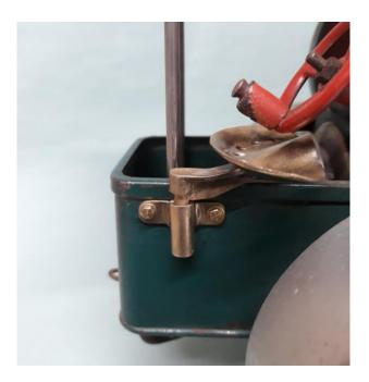
If option (2) then drill through the two holes in the bracket on the rear and bolt in place
